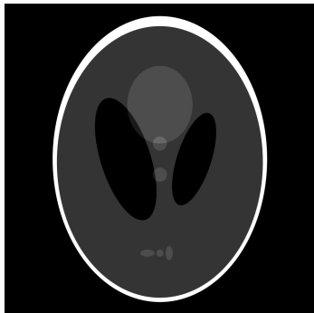
Shepp–Logan phantom: a standard test image.
